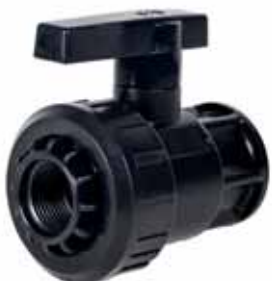
Valve from PP, handle from ABS. PN 10
